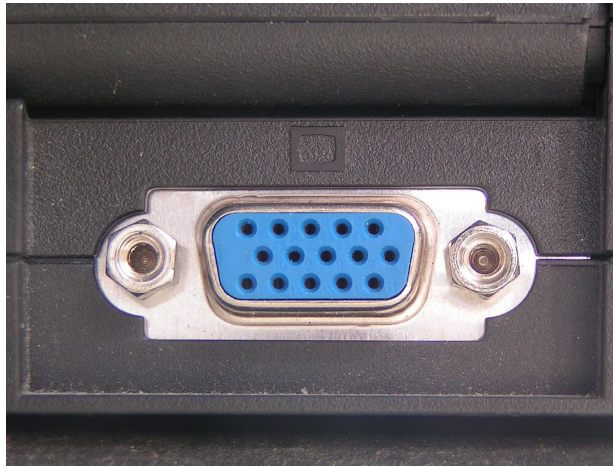
A female DE-15 output in a laptop computer.
