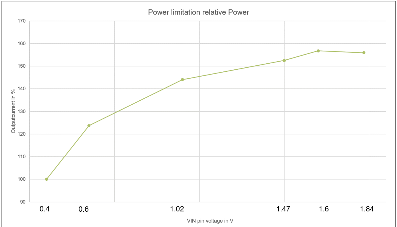
Figure 17 Exemplary representation of the power limitation versus input voltage
